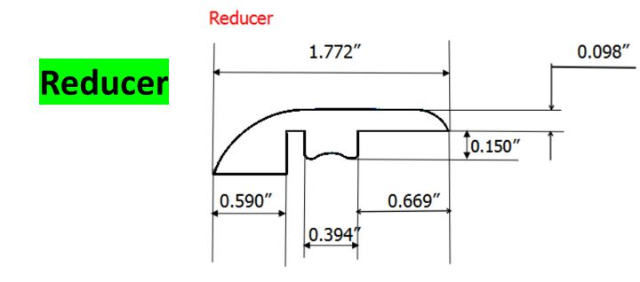
**Tips:** The Reducer molding is the solution in locations where flooring of different heights meet together and a gentle slope is needed to bridge the two surfaces. 100% Waterproof PVC construction.
