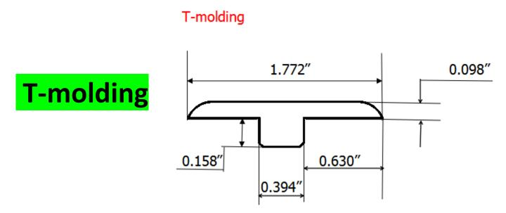
**Tips:** This molding serves to cover the expansion gaps needed in a floating floor installation by bridging the space between two even surfaces. The low profile height and width bring a polished look to the job. They are highly wear resistant and 100% waterproof.
